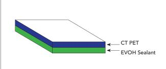
**DESCRIPTION:** Clear pouch film designed for pouch applications which require good barrier properties. The corona treated PET surface provides good ink adhesion for surface printing and good adhesive bond for surface lamination applications. With excellent puncture resistance. This pouch film is an ideal choice for durable pouch applications where barrier properties are required.
